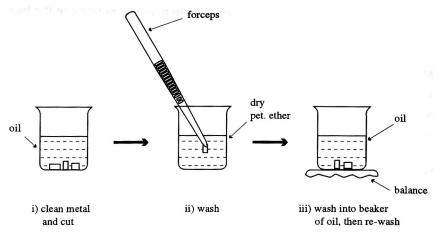
Figure 12: Weighing reactive metals.
