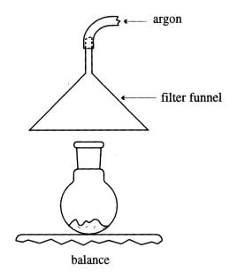
Figure 14: Weighing pyrophoric powdered solids.
