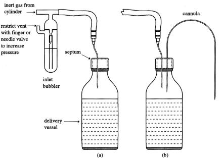
Figure 7: Preparation for a cannula transfer.
