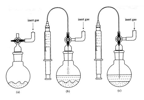
Figure 13: Removing the oil from a dispersion.
