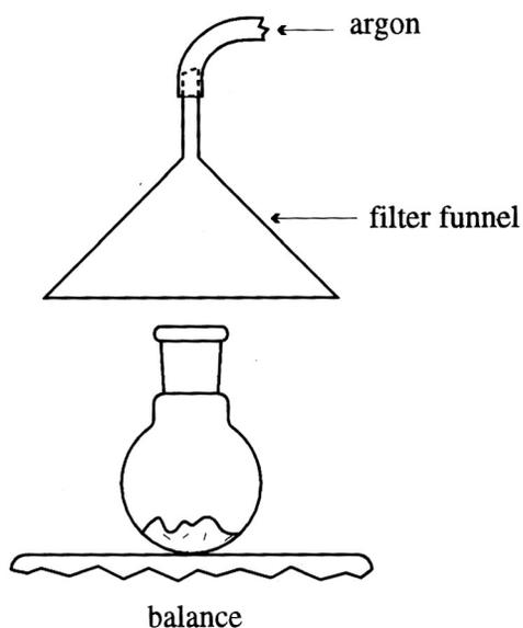
**Figure 14:** Weighing pyrophoric powdered solids.
