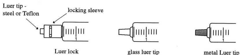
**Figure 4:** Luer lock tip should be used to transfer pyrophoric reagents.
