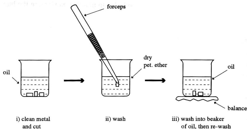
**Figure 12:** Weighing reactive metals.
