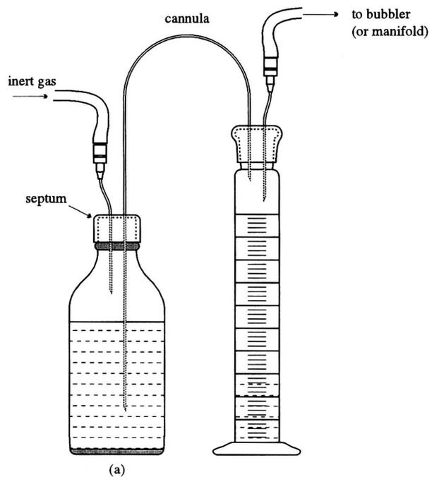
**Figure 9:** Cannulation into a graduated cylinder.
