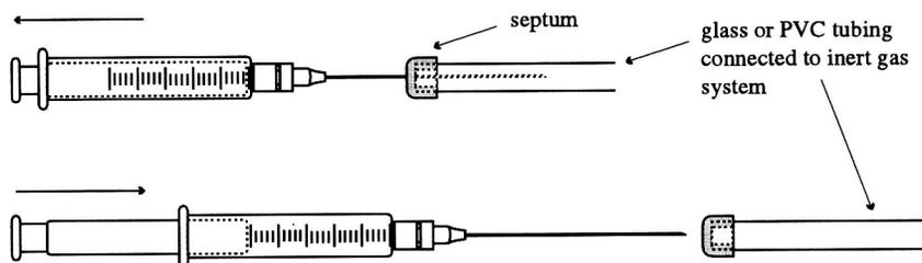
**Figure 5:** The purging of a syringe with inert gas.
