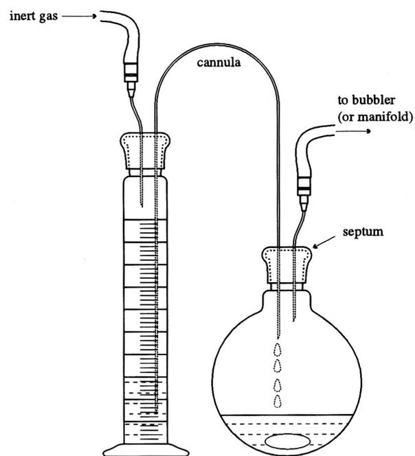
**Figure 10:** Cannulation of a measured volume of liquid.
