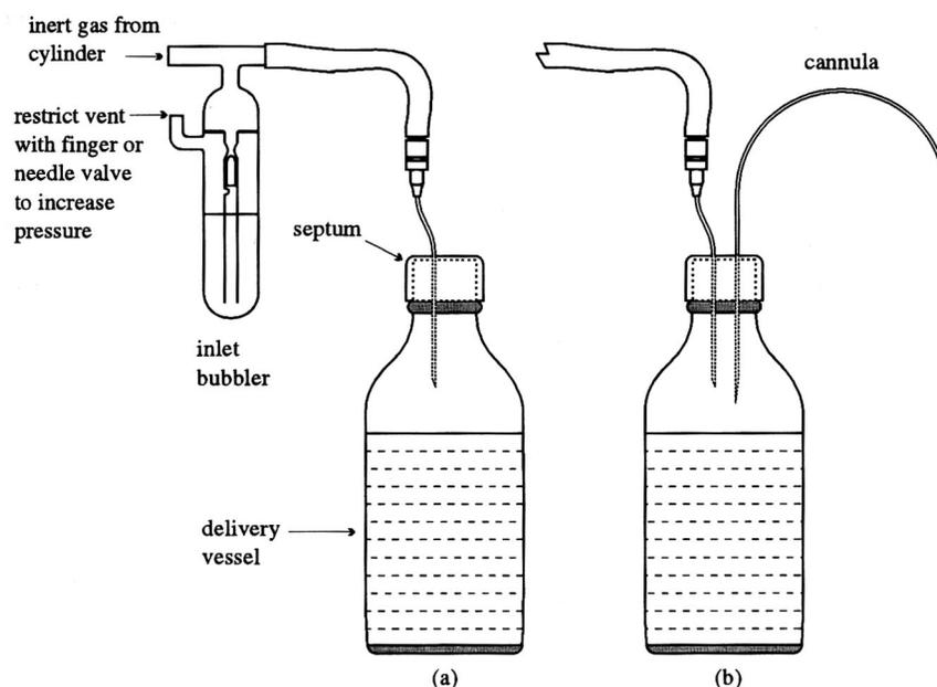
**Figure 7:** Preparation for a cannula transfer.
