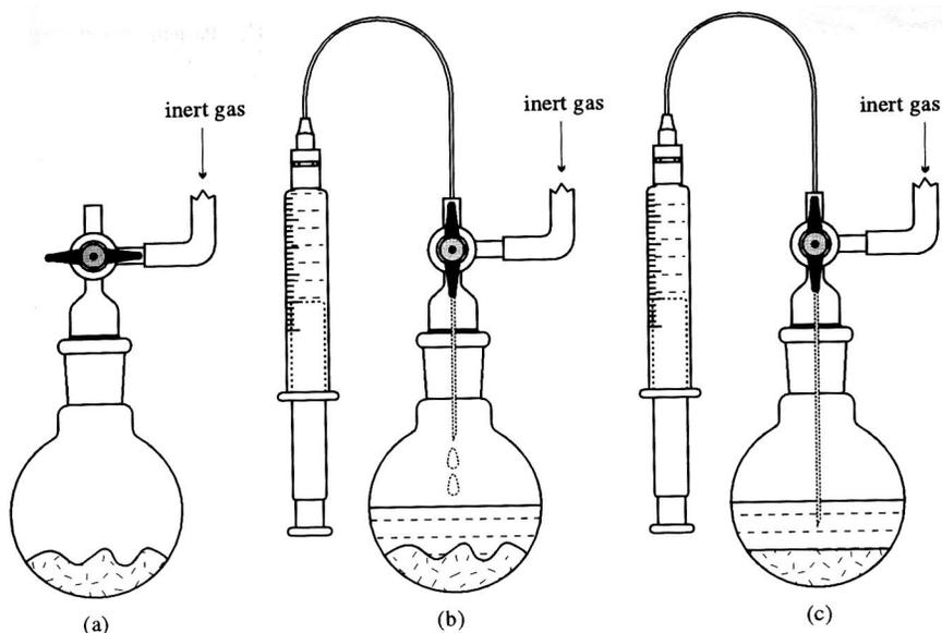
**Figure 13:** Removing the oil from a dispersion.
