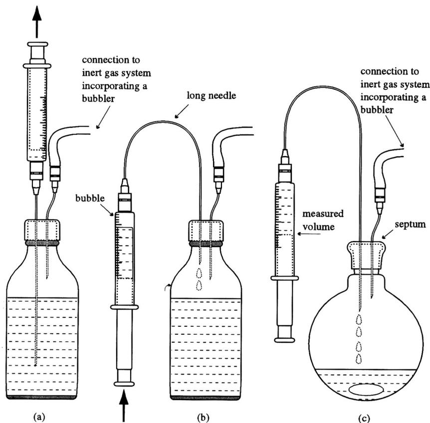
**Figure 6:** Syringe transfer of a pyrophoric reagent.
