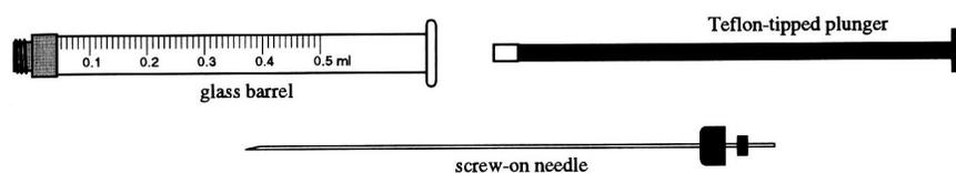
**Figure 2:** A gas-tight microliter syringe.
